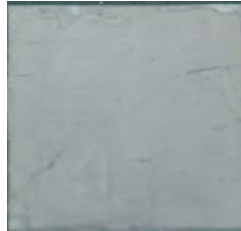
Grease on rear surface
