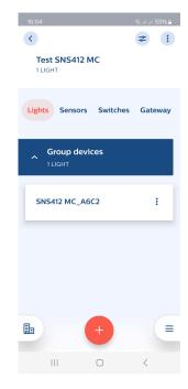
EasyAir SNS412 MC parameters can be configured via Philips MasterConnect App.
