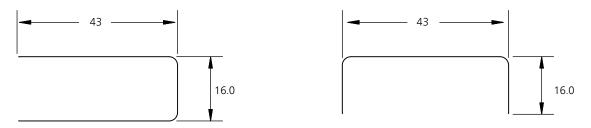
Mounting in cut-out in sheet matal (thickness 0.7 mm to 1.2 mm), tolerance  $\pm$  0.2 mm
