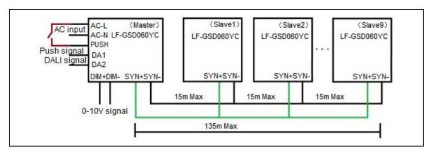
Before using synchronous dimming function, please make sure that all LED drivers are at 100% output.
