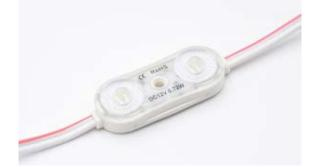
Designed for channel letter illumination in signage applications, the PWM4417-2SLY2835x module is suitable for 3-16cm depth letter illumination & provides bright and even illumination. Supplied in pre-wired chains of 20 pcs with 100mm link wires. Fixing is facilitated by 3M adhesive tape.
