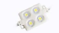
Designed for channel letter illumination in signage applications, the PWM5132 module provides bright and even illumination. Supplied in pre-wired chains of 20 pcs with 78mm link wires. Fixing is facilitated by a 3.6mm hole and 3M adhesive tape. Suitable for 8  $\sim$  18cm depth signs such as channel letters, metal letters, light boxes, decoration, etc
