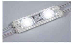
Designed for channel letter illumination in signage applications, the PWM5316-2YL2835x module is suitable for 3-16cm depth letter illumination & provides bright and even illumination. Supplied in pre-wired chains of 20 pcs with 140mm link wires. Fixing is facilitated by 3M adhesive tape.
