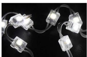
Designed for channel letter illumination in signage applications, the PWM9607-1YL2835T module is suitable for 3-10cm depth letter illumination & provides bright and even illumination. Supplied in pre-wired chains of 100 pcs with 28mm link wires. Fixing is facilitated by 3M adhesive tape.
