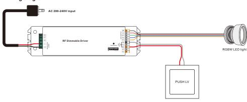
Note: When paired to a single color RF remote and 4 PWM output channels are wired to LED loads simultaneously, please make sure the operation current of the LED loads does not exceed 1100mA.
