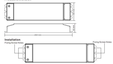
Note: when mounting the driver, please choose any one of the three fixing screw holes to fix with a screw at each end.
